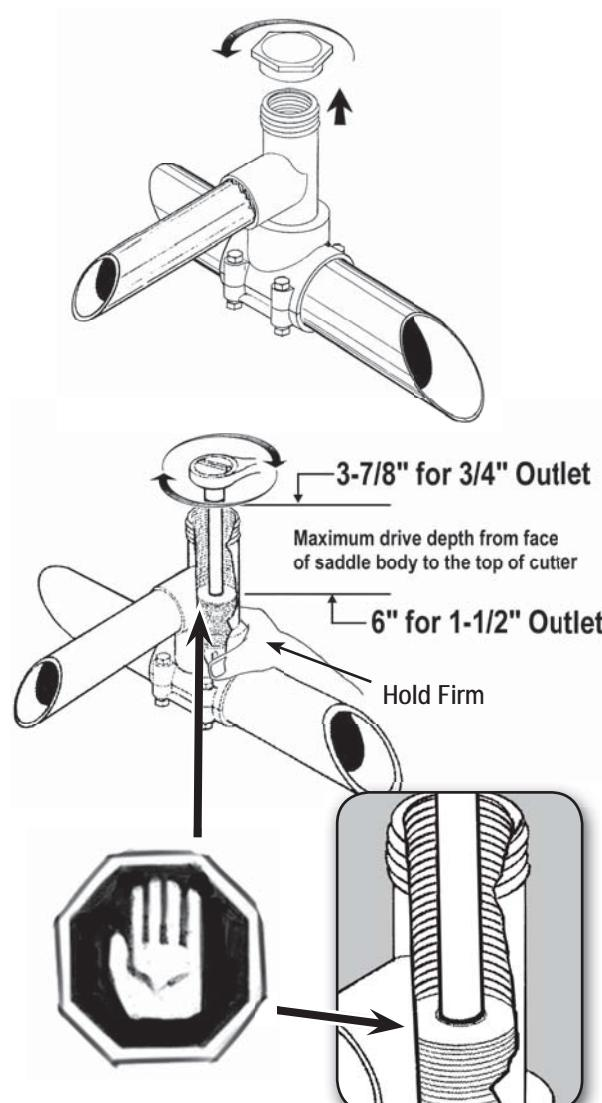
Resistance will occur when the blade contacts the pipe. Continue until resistance is reduced, indicating that the cutter has cut through the pipe.
