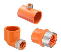
SPEARS® Patented Special Reinforced (SR) plastic female thread design is one of the most significant advancements in the use of CPVC Fire Sprinkler System threaded fittings. Not just an added ring, this unique precompression design compensates for expansion forces generated from tapered pipe thread joint make-up. Radial stress is no longer a problem in normal installations and easily managed in severe over-tightening situations.
